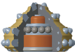
滑动轴承橡胶密封 Rubber Sealed Sliding Bearing
